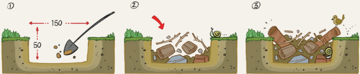
At a minimum excavate a hole 50cm deep and 150cm wide.
